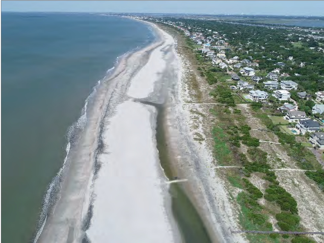
FIGURE 4.19. By being positioned downdrift of the nourishment area, Reach 4 receives nourishment sand spreading from the placement area as well as spreading shoal sand. This reach has gained sand every year since 2009 except 2016.
