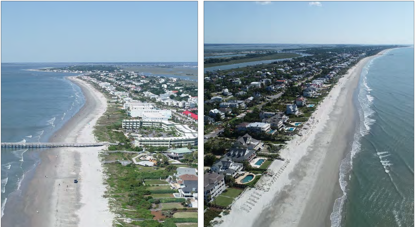
FIGURE 4.28. Aerial views of Reach 2 in June 2020. Since monitoring began in 2009, Reach 2 has been the most stable reach, typically showing lower magnitudes of volume change compared to the other reaches along Isle of Palms. The arc in the shoreline west of the pier indicates that the pier may act to trap sand, which may impact Reach 2 in certain wave conditions.
