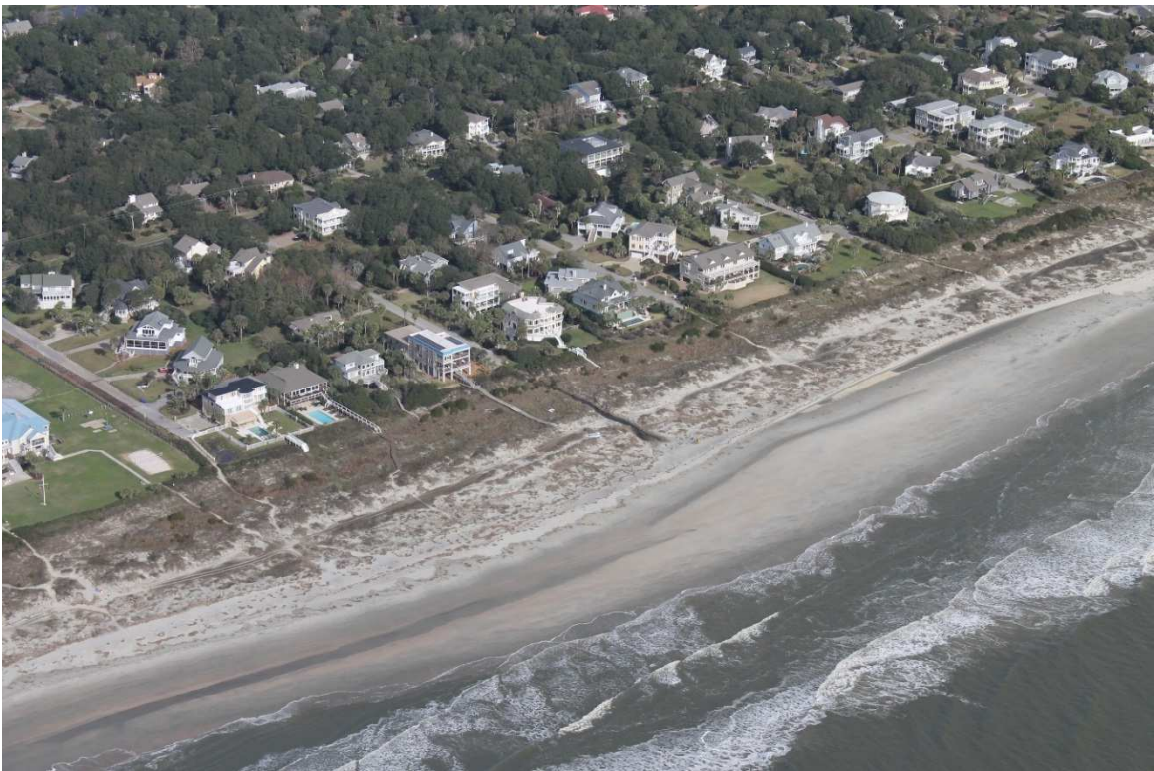
FIGURE 3.32. January 2016 photos of Reach 4. The lower photo shows the 49th Avenue beach access which was washed out during Hurricane Joaquin . The waviness of the dry-beach line reflects natural variations in the orientation, position, and width of intertidal sand bars. Sediment tends to move downcoast (right to left as viewed here) in “packages” rather than at a steady rate which would yield a straighter shoreline.
