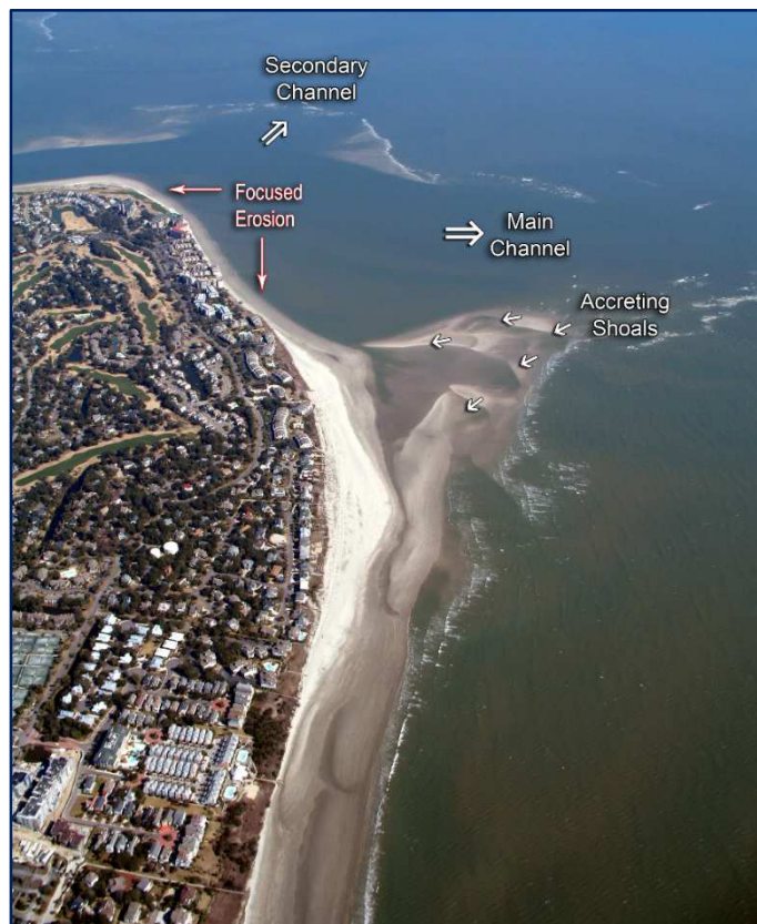
FIGURE 1.5. 2007 aerial image of the northeast end of Isle of Palms, showing a large shoal event attached to the beach.
