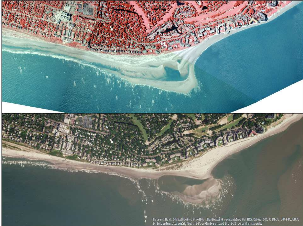
FIGURE 3.24. Aerial images of shoal attachments from 2007 and 2015. The 2015 event is attaching further east than the 2007 event, resulting in different portions of the beachfront experiencing focused erosion. [Upper image by IMC, Charlotte NC and lower image via ESRI World Imagery]
