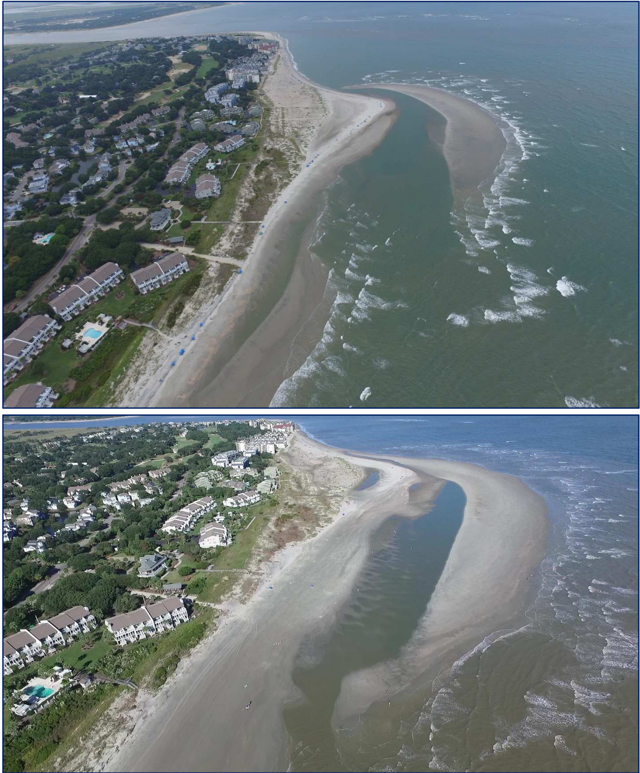
FIGURE 3.5. August 2015 (upper) and October 2015 (lower) aerial images of the attaching shoal at the northeast end of Isle of Palms. The center of the shoal (top of images) stalled between 2014 and August 2015, but moved onshore during Hurricane Joaquin .
