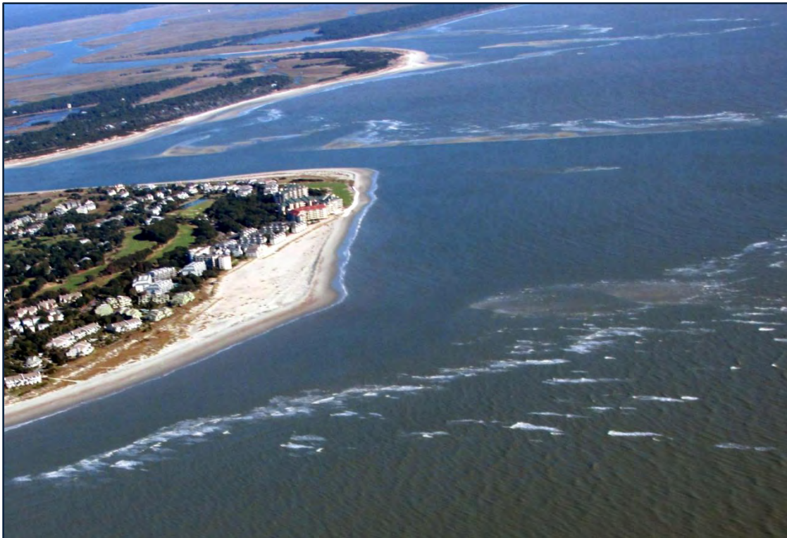
FIGURE 3.44. July 2013 (upper) and November 2013 (lower) aerial images of the ongoing shoal-bypass event at the northeastern end of Isle of Palms. It is apparent that the main body and western area of the shoal have migrated closer to the beach since July (date of survey data). [Note the November image was taken at a slightly higher tidal stage, reducing the extent of the breakers and area of exposed sand.]
