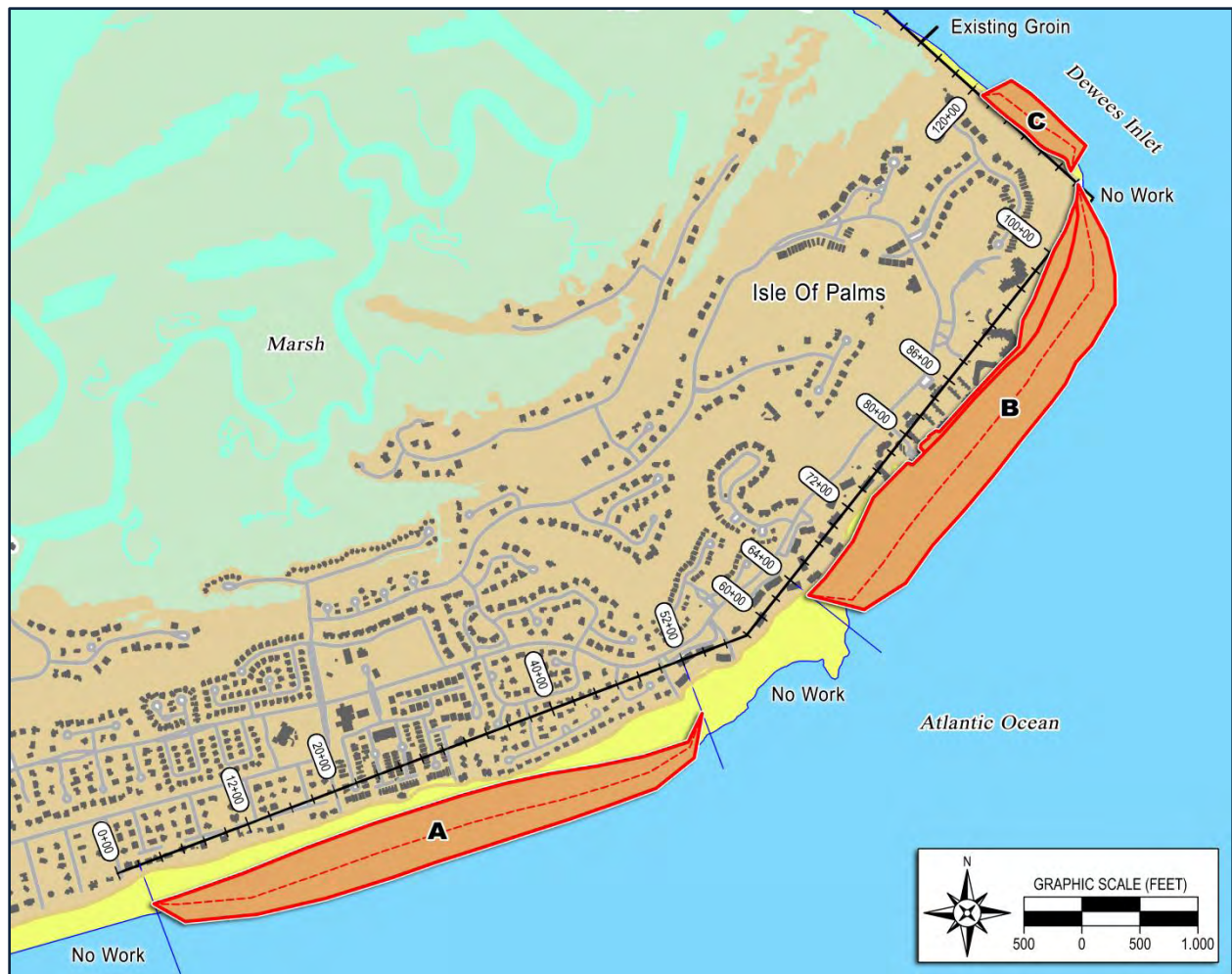
FIGURE 3.45. Reaches for the 2008 nourishment project. The graphic shows the project baseline with 0+00 located at 53 rd Avenue (monitoring station 222+00).
