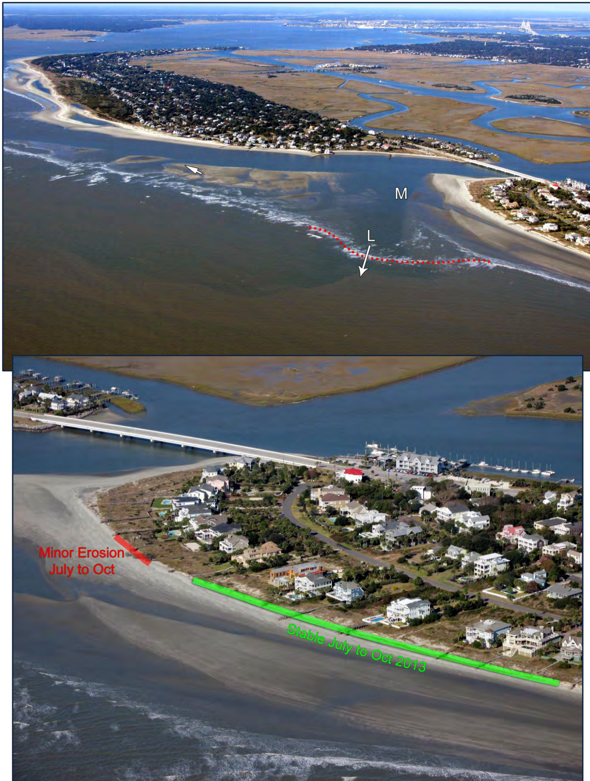
FIGURE 3.37. November 2013 aerial images of Breach Inlet area. [UPPER] View of the Breach Inlet delta, which extended southwest (toward Sullivan’s Island) from 2012 to 2013, likely drawing sand off the IOP beach. The marginal flood channel (M) migrated toward the beach and developed a terminal lobe (L) through the delta shoal. [LOWER] View of the western tip of Isle of Palms showing areas which were stable or erosional between July and October 2013. While a small area showed minor dune recession, all stations in this view gained sand from July to October 2013 (measured to -6 ft NAVD). [Photos by SB Traynum]
