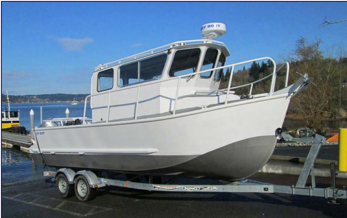
FIGURE 2.2. CSE beach monitoring methods include land-based data collection using Trimble™ RTK GPS from the backshore to low-tide wading depth and over-water work using RTK GPS linked to a precision echosounder aboard CSE's survey boat (RV Southern Echo ).
