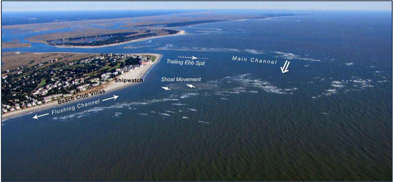
FIGURE 3.17. November 2013 oblique aerial image of the northeastern end of Isle of Palms. Several events are occurring simultaneously, all of which have an impact on the beach condition. CSE expects the beach will evolve rapidly over the next year due to the current shoal-bypass event.
