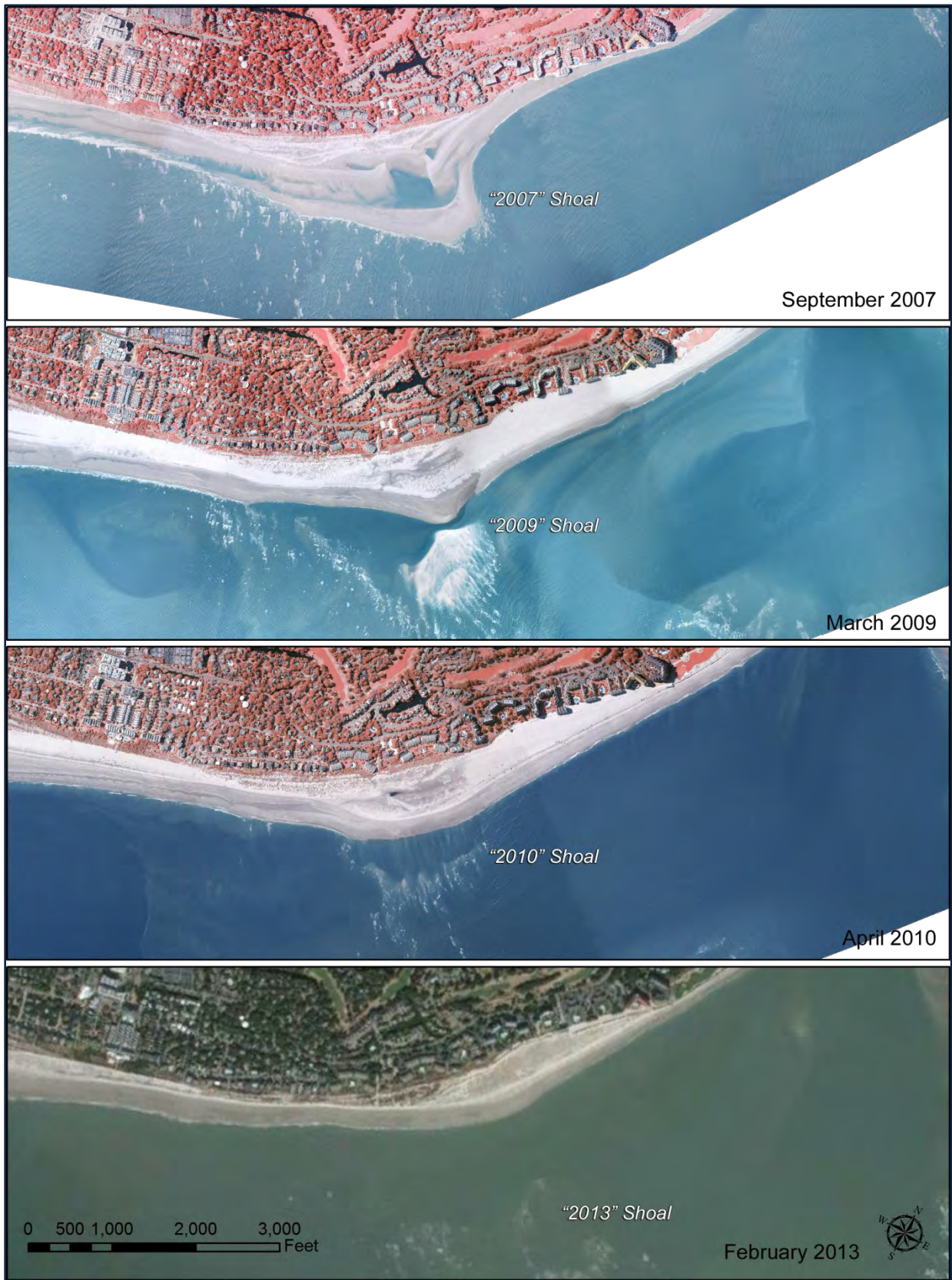
FIGURE 3.10. Sequence of aerial photographs showing four distinct shoal-bypass events occurring between 2007 and 2013. The 2009 and 2010 events were of much smaller scale than the 2007 event or the present event. The first three images were obtained by Independent Mapping Consultants (IMC, Charlotte NC); the fourth image was obtained from Google Earth (2013).
