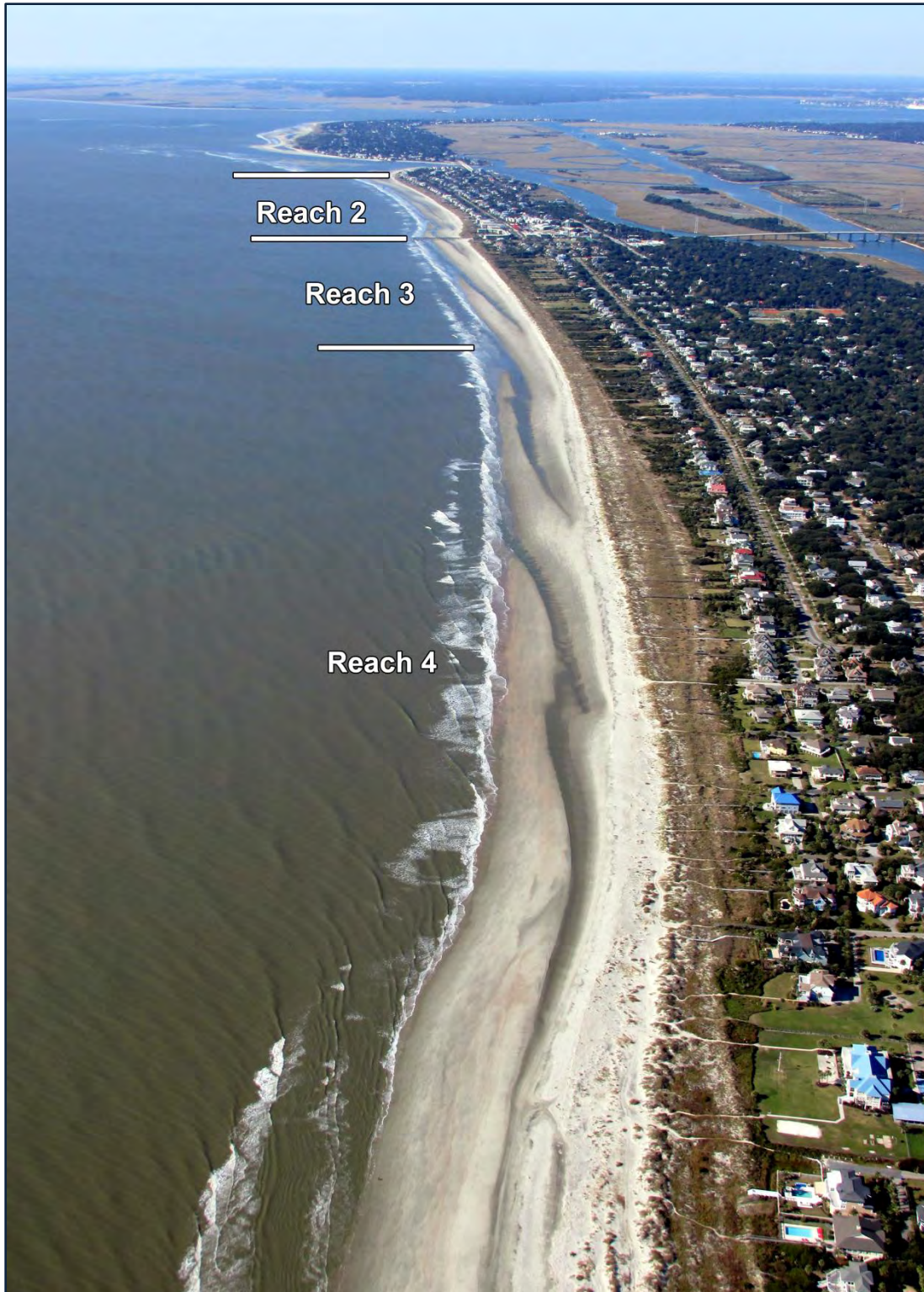
FIGURE 3.27. November 2013 aerial image of the central portion of Isle of Palms. Steady long-term accretion has resulted in wide vegetative buffers and protective dunes. Note oblique low-tide bars and troughs (“runnels”) along the beach, which form under the influence of waves from the northeast. [Photo by SB Traynum]
