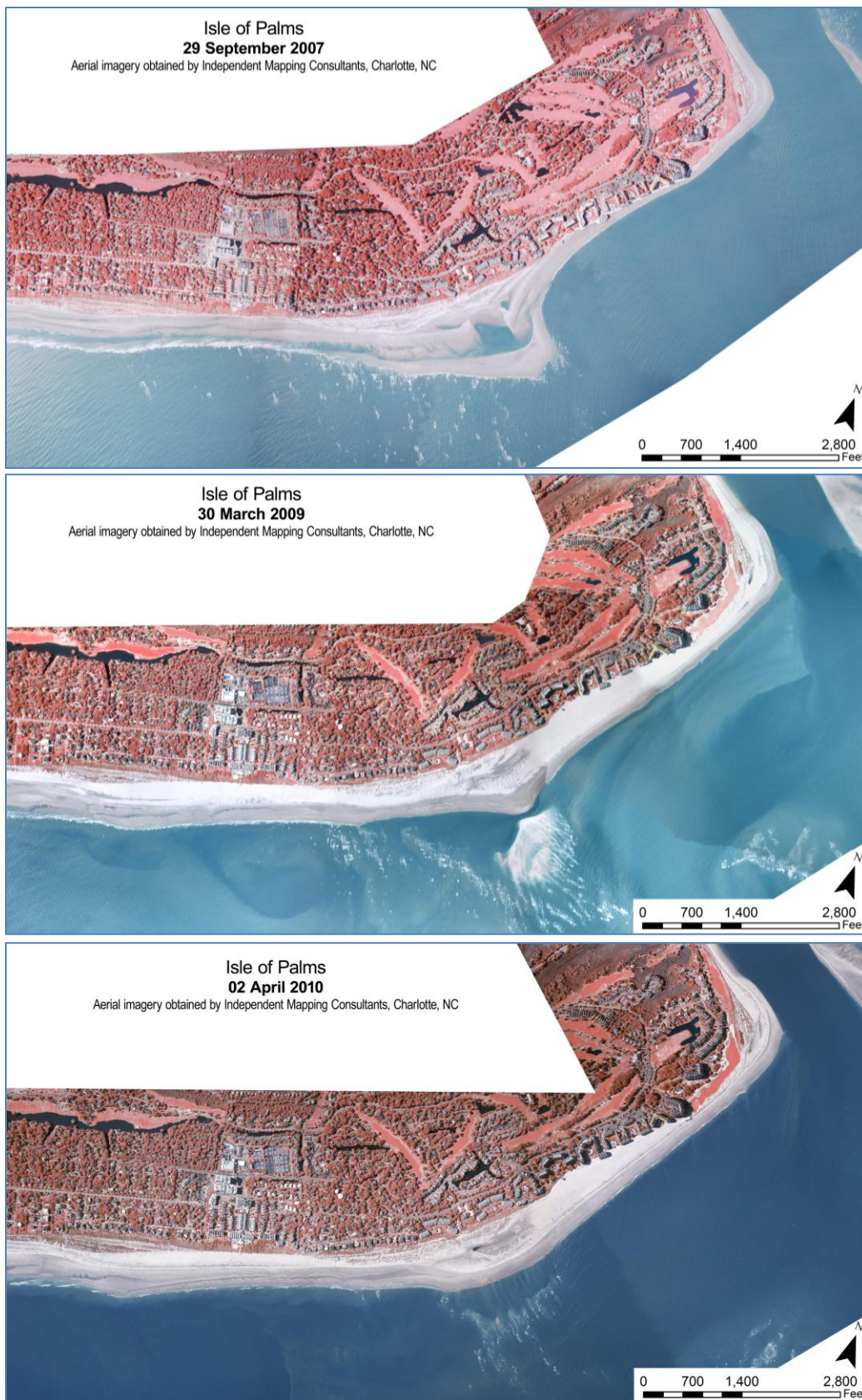
FIGURE 3.14. Reach 5 and Reach 6 in September 2007 (upper), March 2009 (middle) and April 2010 (lower). Note the erosional arc in the 2007 image adjacent to the Wild Dunes Grand Pavilion (left center of image). The “2008” shoal is visible in the middle image, and the “2010” shoal in the lower image. [See Figure 3.34 for 2011 image.]
