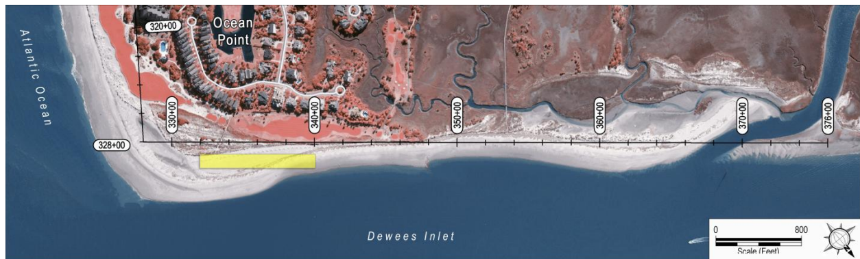
FIGURE 3.3. Station map of the Dewees Inlet area (Reach 7). Reach 7 spans from station 330+00 near the 18 th tee to station 368+00 near Cedar Creek spit. The approximate limits of nourishment Reach C are identified by the yellow bar. The 1981 low profile groin is positioned near station 348+00. [March 2009 aerial image by Independent Mapping Consultants Inc]
