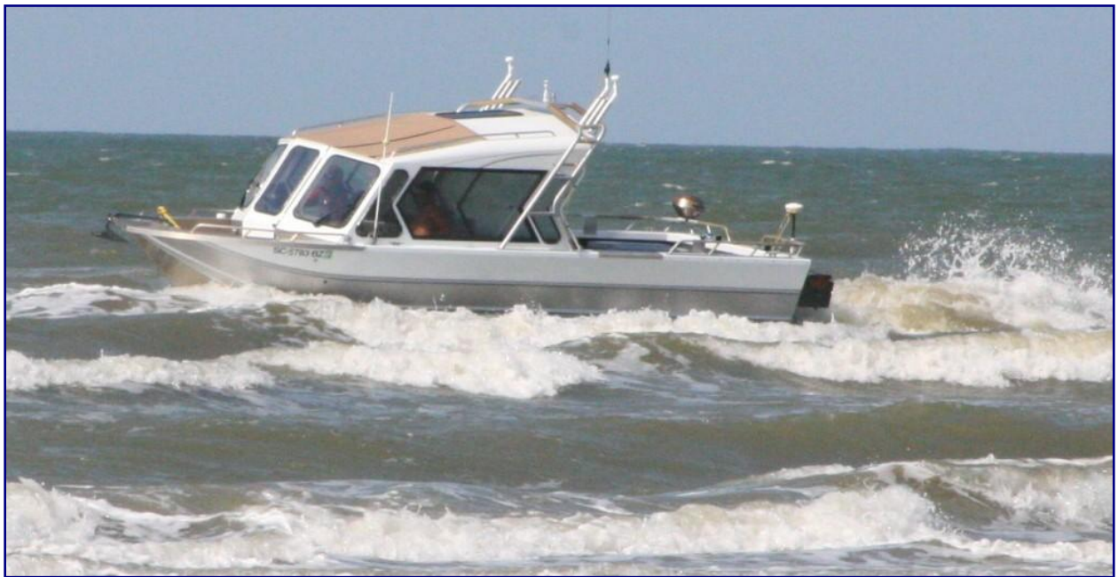
FIGURE 2.2. CSE beach monitoring methods include land-based data collection using Trimble™ RTK GPS from the backshore to low-tide wading depth and over-water work using RTK GPS linked to a precision echosounder aboard CSE's shallow draft boat (RV Congaree River).
