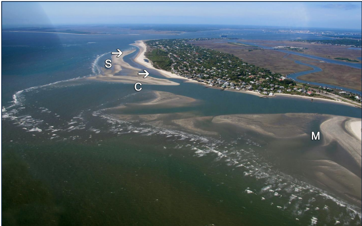
FIGURE 3.32. Aerial image of Breach Inlet taken 15 April 2011 (TW Kana). A channel (C) avulsion has triggered a large shoal-bypass event on Sullivan’s Island (S). The new main channel is oriented more perpendicular to the shoreline. Only a minor remnant of a marginal flood channel (M) was present on the Isle of Palms side when this photo was taken.
