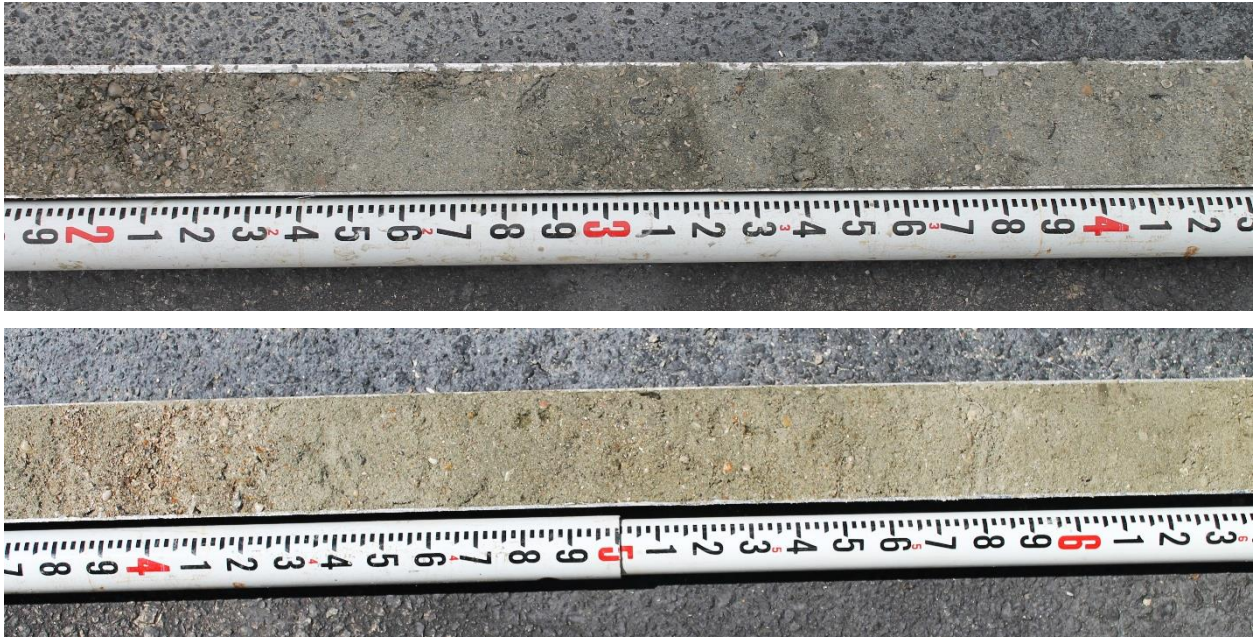
Figure 2. Photos of typical borings from Areas E and F (upper) and the offshore areas in the proposed historic district (lower). Note the sand in the lower boring is more tan, and contains less silty material (as visible in the darker areas in the top photo).
