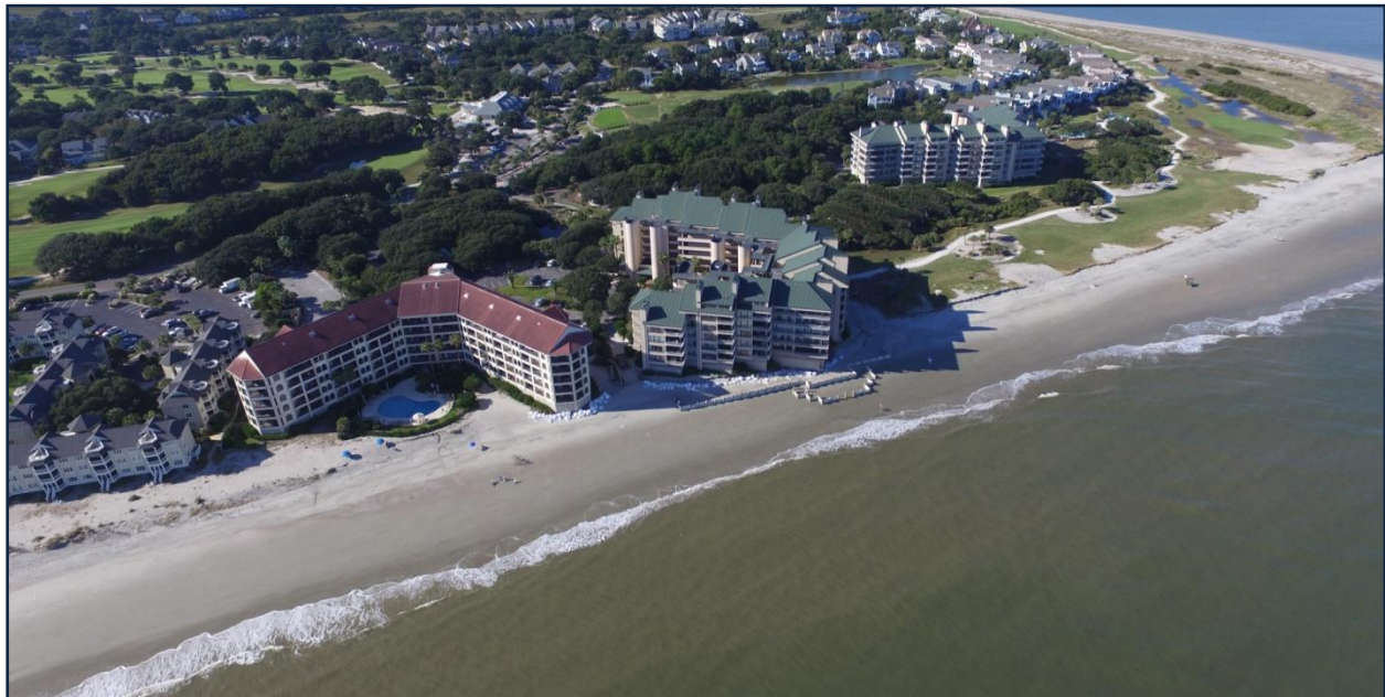
FIGURE 7. October 2015 post-storm aerial images of the area near Seascape and Ocean Club. The intertidal beach width is narrow in front of Ocean Club, limiting the availability and practicality of emergency sand scraping.
