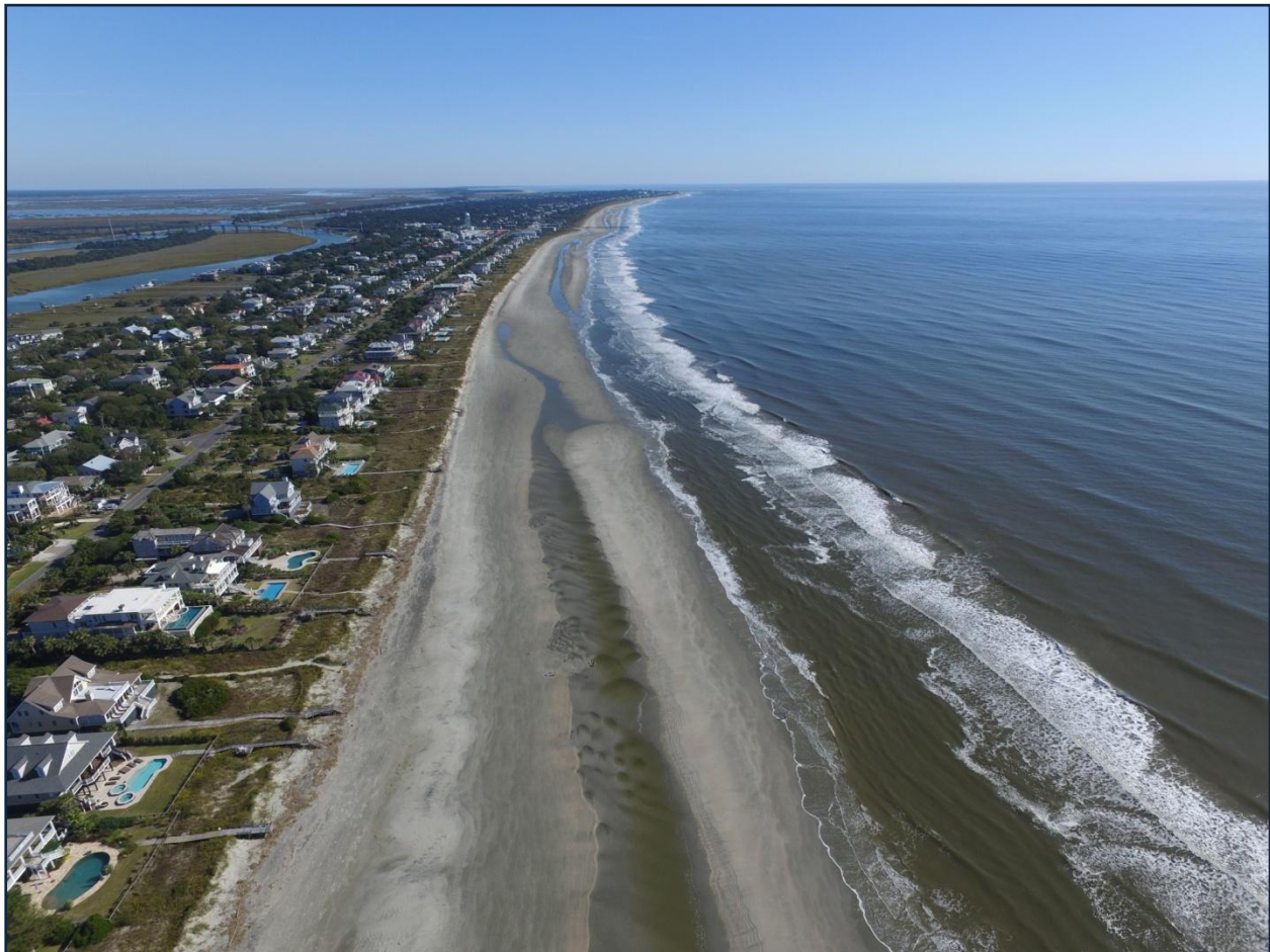
FIGURE 8. October 2015 post-storm aerial images of the area between Breach Inlet and Front Beach. The intertidal beach width is wide in this area, despite an erosional arc centered at 5 th Avenue. Emergency sand scraping may be beneficial in restoring the eroded primary dune.
