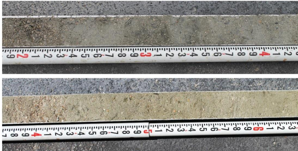
Figure 2. Photos of typical borings from Areas E and F (upper) and the offshore areas in the proposed historic district (lower). Note the sand in the lower boring is more tan and contains less silty material (as visible in the darker areas in the top photo).
