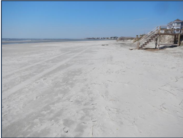
April 2014 images from station 20+00, looking west (left) and landward (right). Despite a net loss of 10 cy/ft at the station (January–April), the dry beach accreted and the old escarpment continues to heal.
