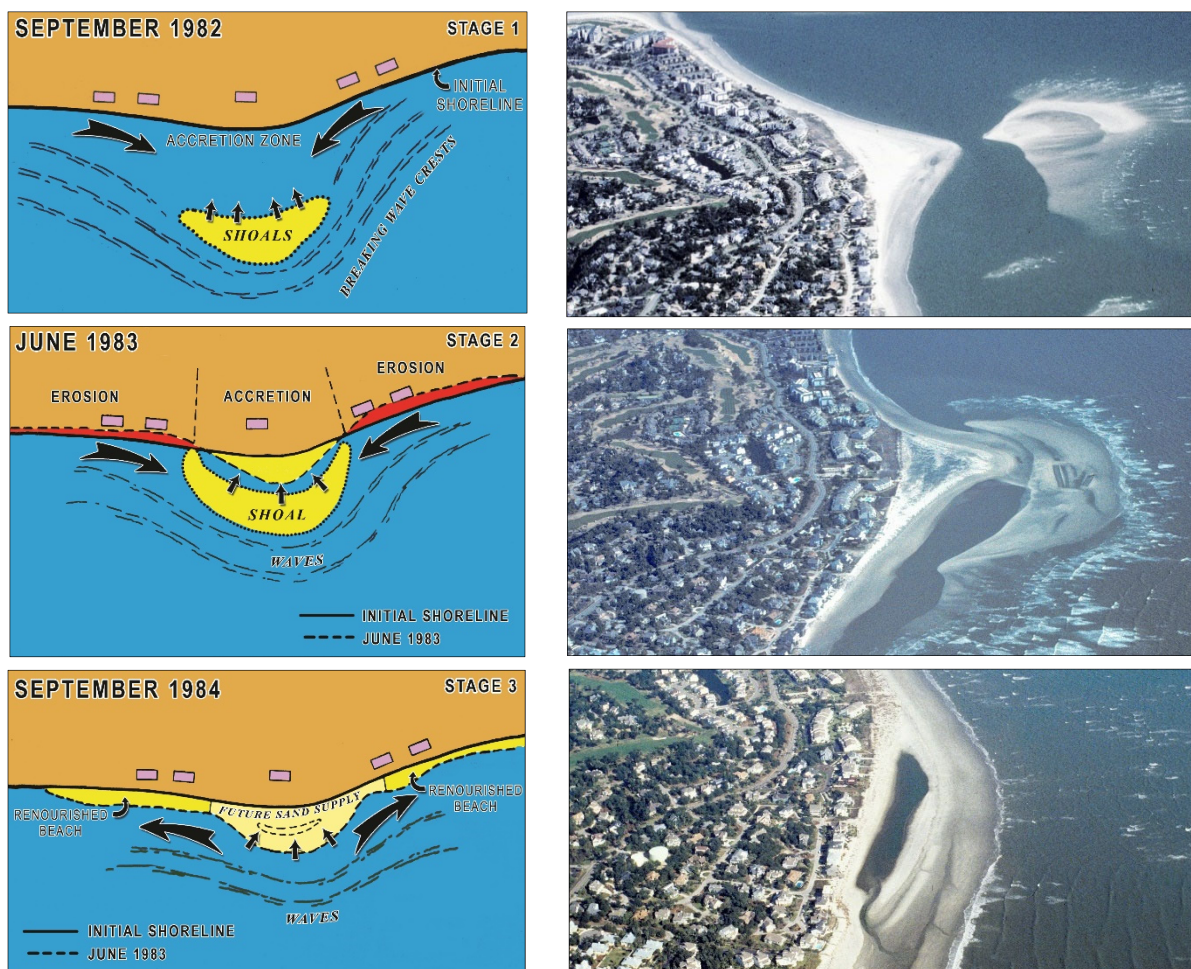
FIGURE 2.3. [LEFT] Schematic of the shoal-bypass cycle originally modeled from a bypass event at Isle of Palms. [RIGHT] A shoal-bypass event at northeastern Isle of Palms corresponding to the schematic. The upper photo shows a shoal in Stage 1 (1996). The middle image illustrates Stage 2 (1997). The bottom photo shows Stage 3 (1998).
