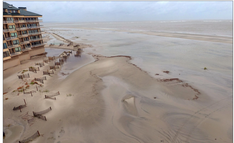
FIGURE 4.11. Aerial photos of Reach 6 following Hurricane Dorian in September 2019 which document significant overwash of the berm.
