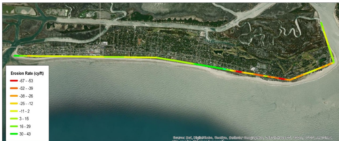
FIGURE 4.1. Line map showing erosion and accretion patterns over Isle of Palms from April 2019 – July 2021.
