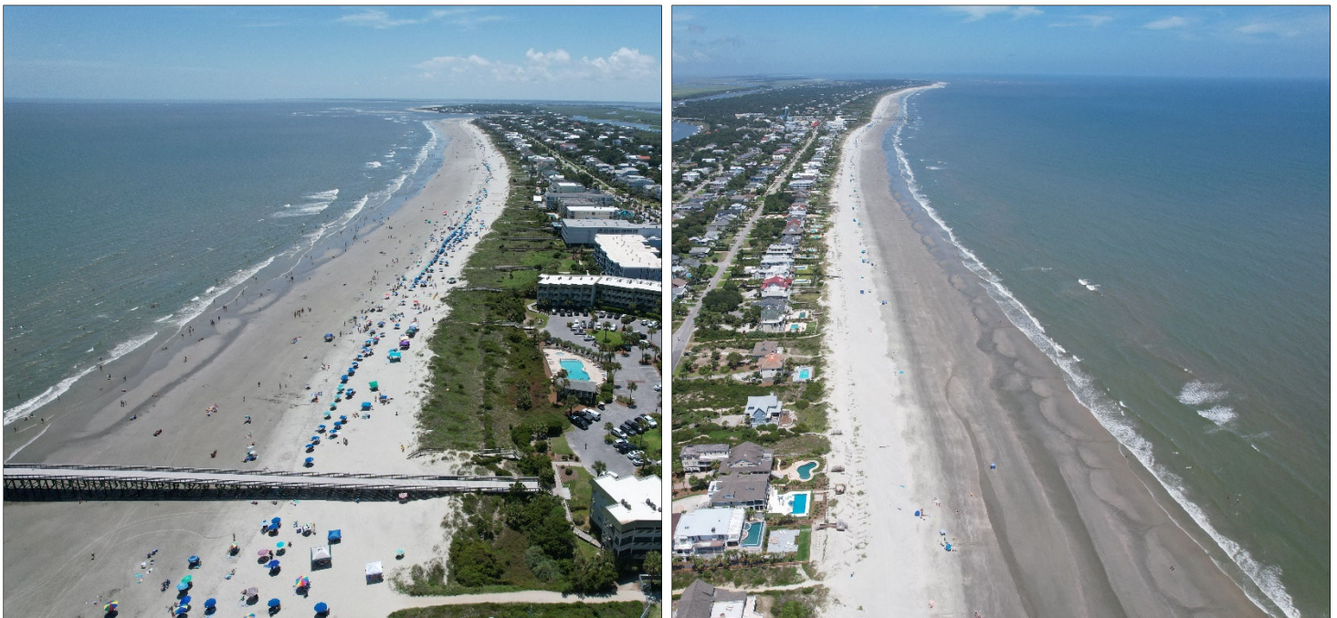
FIGURE 4.26. Aerial views of Reach 2 in July 2021. Since monitoring began in 2009, Reach 2 has been the most stable reach, typically showing lower magnitudes of volume change compared to the other reaches along Isle of Palms. The arc in the shoreline west of the pier indicates that the pier may act to trap sand, which may impact Reach 2 in certain wave conditions.
