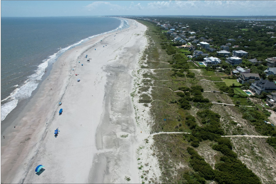
FIGURE 4.18. By being positioned downdrift of the nourishment area, Reach 4 receives nourishment sand spreading from the placement area as well as spreading shoal sand. This reach has gained sand every year since 2009 except 2016. As the vegetated dunes expand, sheltered locations (such as low-lying areas behind protective dune ridges) will gradually transform into a shrub habitat with larger areas of wax myrtle replacing dune grasses.
