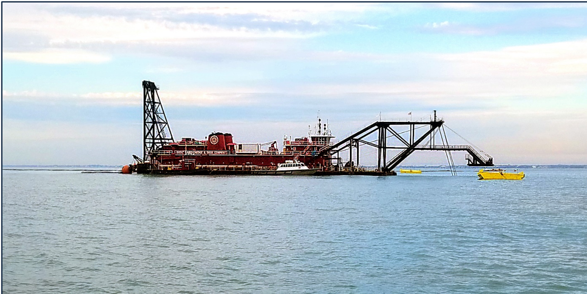
PHOTO 2. Great Lakes Dredge and Dock Company's cutter suction dredge the Illinois digging on borrow area F.
