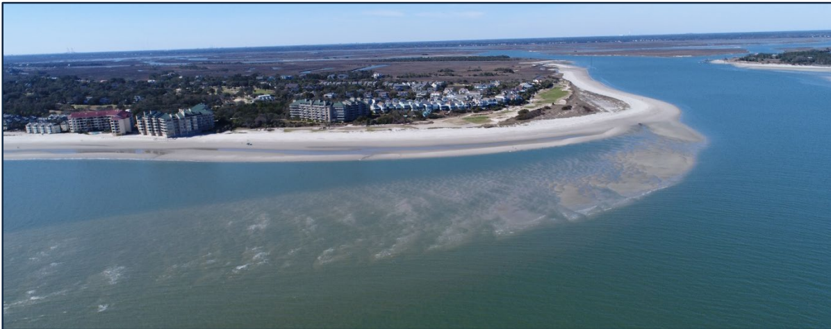
FIGURE 2.14. Trailing-ebb-spit extending from the northeast end of the island on the landward side of the Dewees Inlet channel. Rapid erosion along the eastern end of Reach 6 likely contributed to this event.
