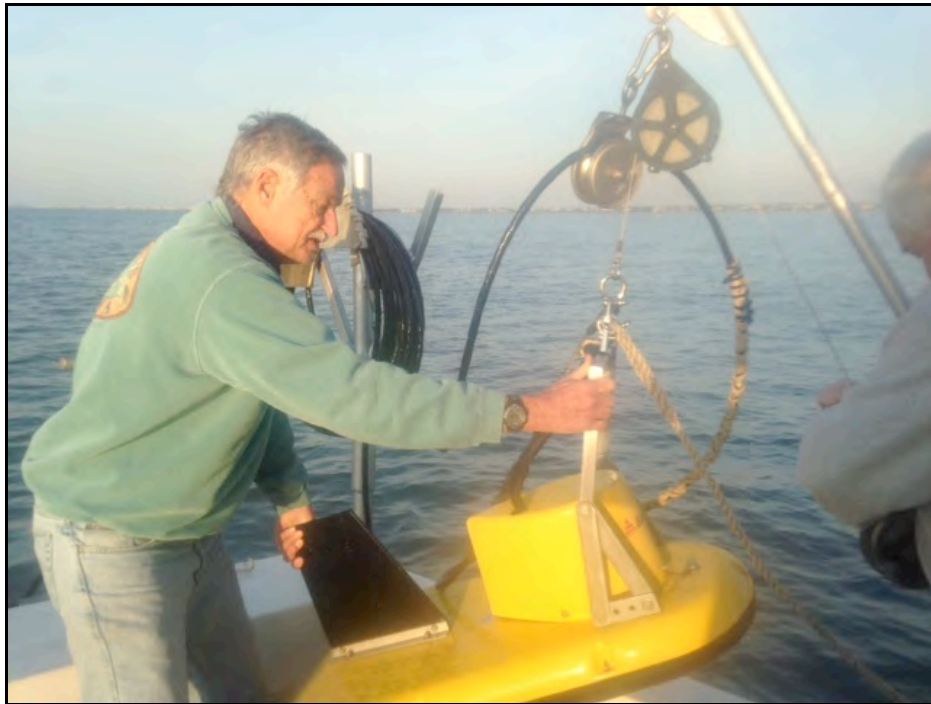
Figure 8. Launching the EdgeTech SB-216S tow vehicle.
