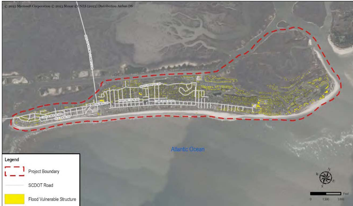
Preliminary structure vulnerability due to intermediate sea level rise projections (3.89 feet) for year 2100.
